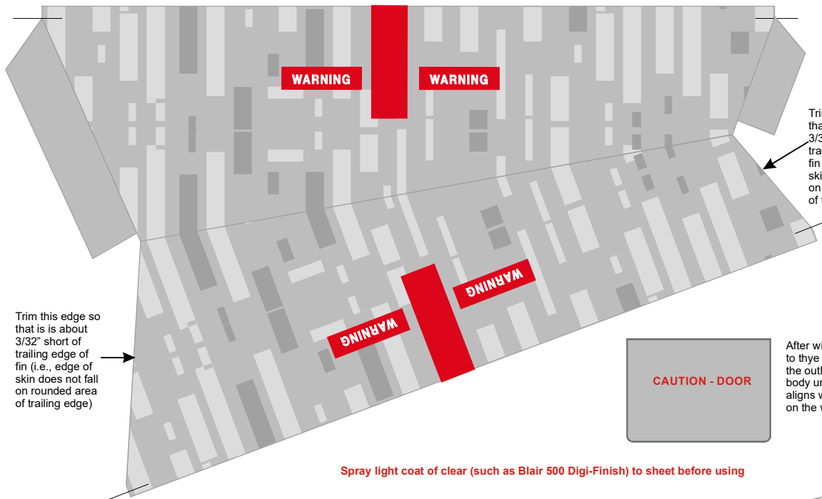
Bottom left wing skin (apply after apply top wing skin)
